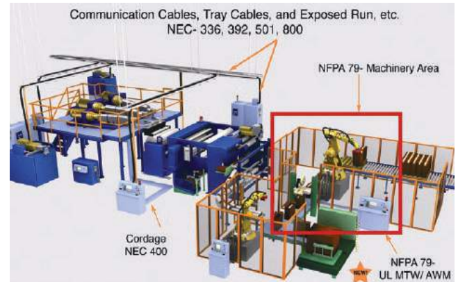
This schematic of an industrial machine shows the main applications of cables and wires with reference to the relevant sections in NEC®/NFPA. “NEC®” is a trademark of the National Fire Protection Association (NFPA).
